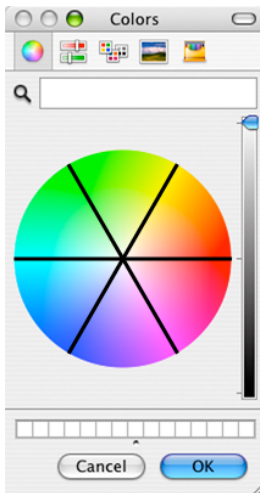
4. Bisecting a color wheel with a straight line defines complements – colors that produce a neutral color when mixed in equal proportions. Increasing one color reduces its complement. Three complementary axes are particularly important in color adjustment – red/cyan (0/180), yellow/blue (60/240), green/magenta (120/300).
