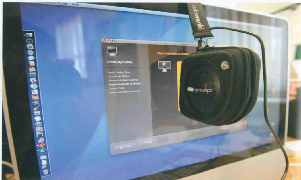
↑ The x-rite ColourMunki in action, hanging off our office iMac in its protective neoprene bag while measuring colour values.
