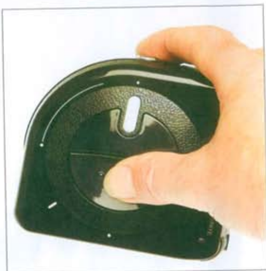
ColorMunki is a robust hand-sized device with three functions – screen calibration, printer profiling, and colour sample measurement.
