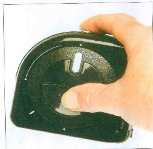
ColorMunki is a robust hand-sized device with three functions – screen calibration, printer profiling, and colour sample measurement.
